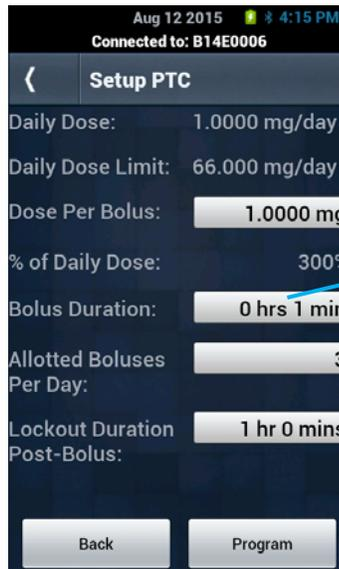
**After first setup, current bolus settings are displayed following successful pump link**
