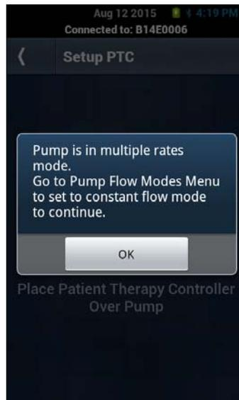
**Unsuccessful link with Pump due to pump not being in Constant Flow Mode**
